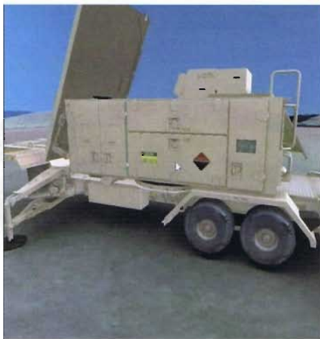
Above 3D courseware – virtual maintenance part-task trainer for the Patriot ballistic missile radar system.
